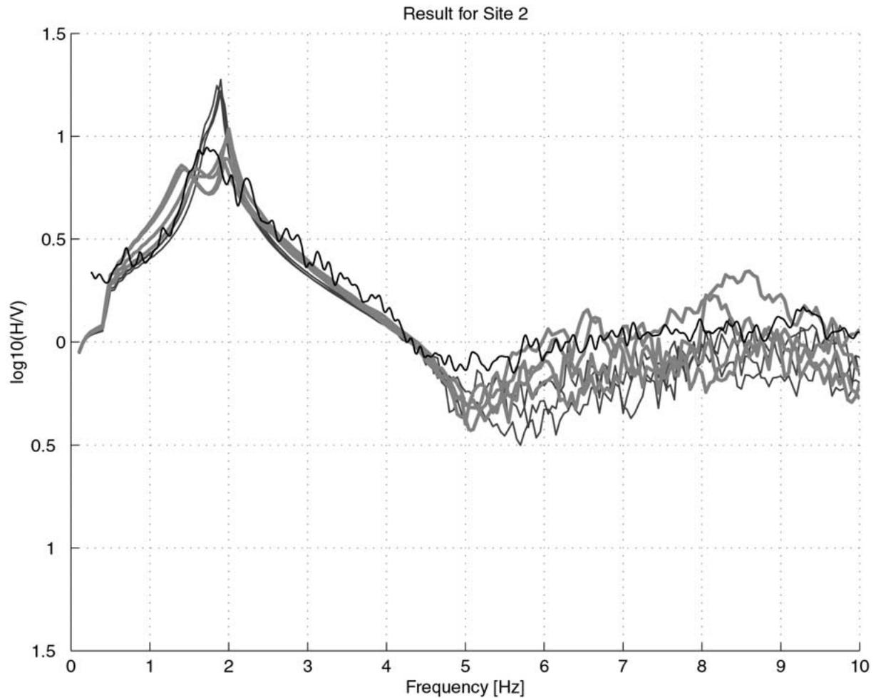
Figure 4. Synthetic H/V ratios (light and dark gray lines) obtained for the inverted structural models in Figure 3B, compared to the observed H/V ratio at observation point No.2 (thin black line).
