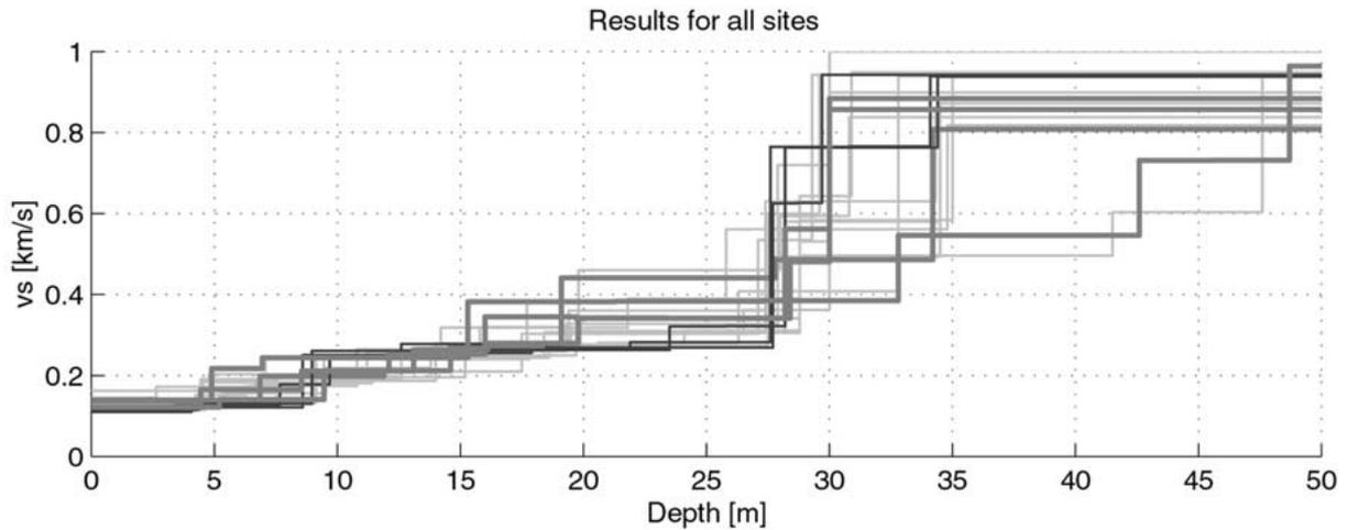
Figure 8. Structural models obtained from the different inversions of the observed H/V ratios (gray lines) at observation point No.2, compared to the inverted models for the other four observation sites shown in Figure 1.
