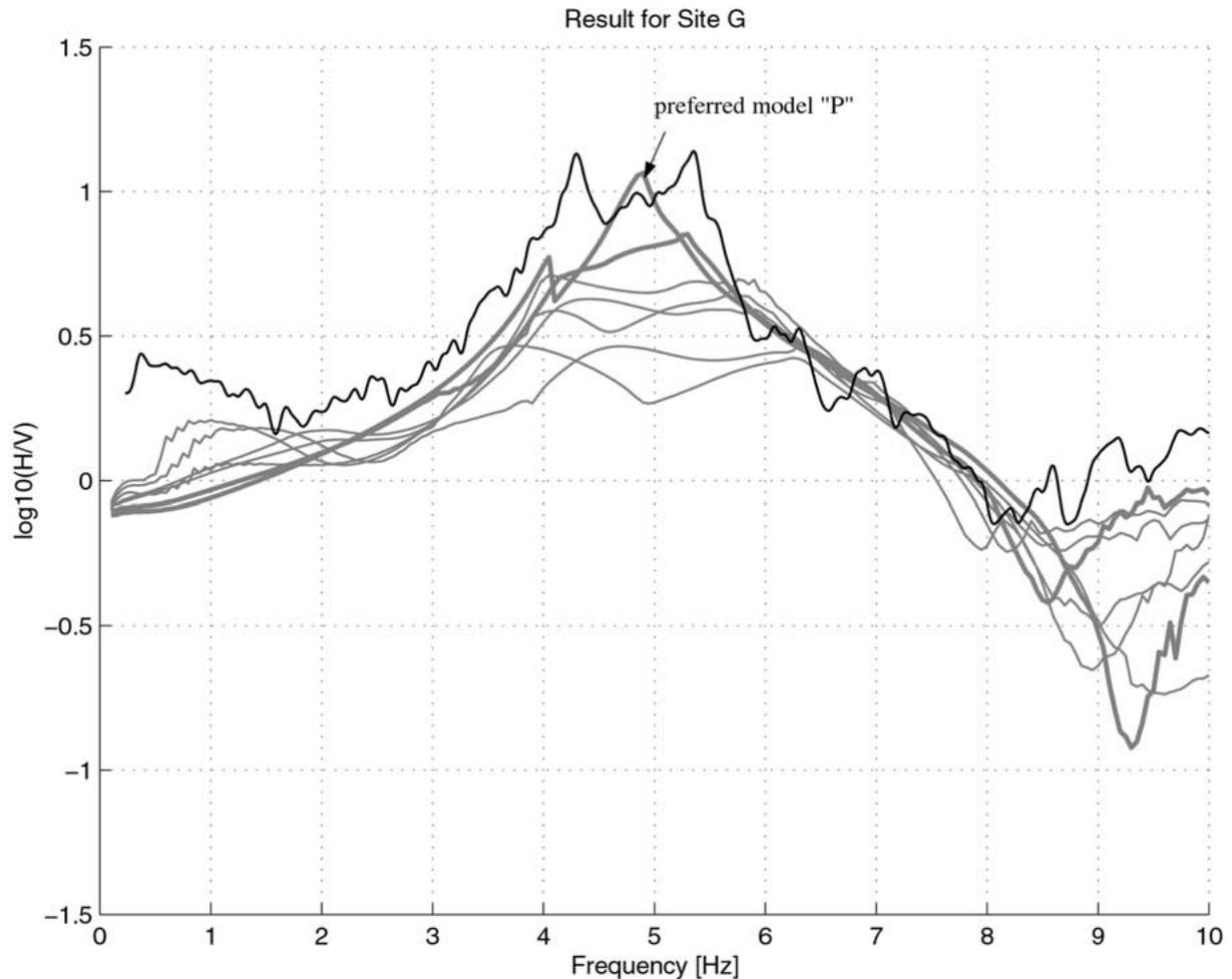
Figure 10. Synthetic H/V ratios obtained for the inverted structural models in Figure 9B, compared to the observed H/V ratio at site G. The result for the preferred model 'P' from the H/V inversion is indicated.
