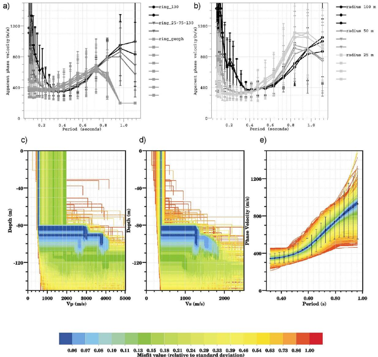
Figure 2: (a) and (b) Dispersion curves obtained at two different times with two different networks. (c) Vp and (d) Vs models resulting from the non linear inversion of the dispersion curve (e).
