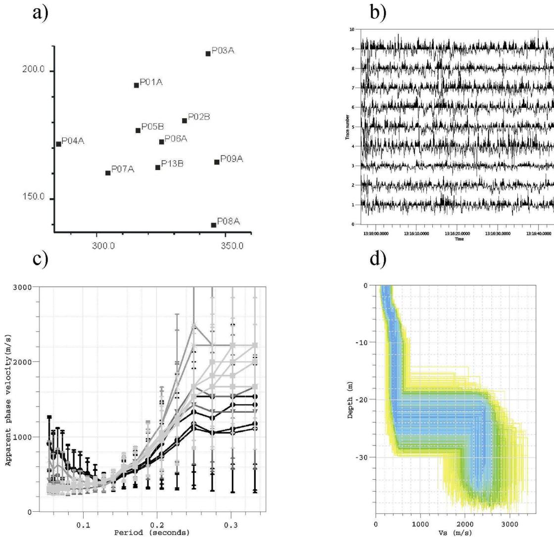
Figure 1: (a) Geometry of the station array. (b) Records of ambient vibrations at the stations. (c) Dispersion curves with error bars for different time windows and array geometries. (d) S-wave velocity profiles explaining the dispersion curves. The darkest models present the lowest misfit values.
